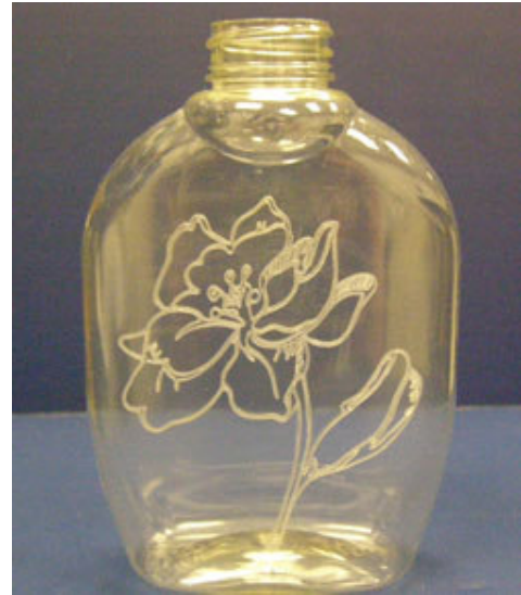
This plastic PET bottle was marked with a 25W laser at a velocity of 40"/second. The flower graphic was completed in a cycle time of 1.80 seconds.
