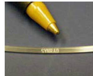
This plastic medical tubing was marked with our 48-1, using just 5W of power.
