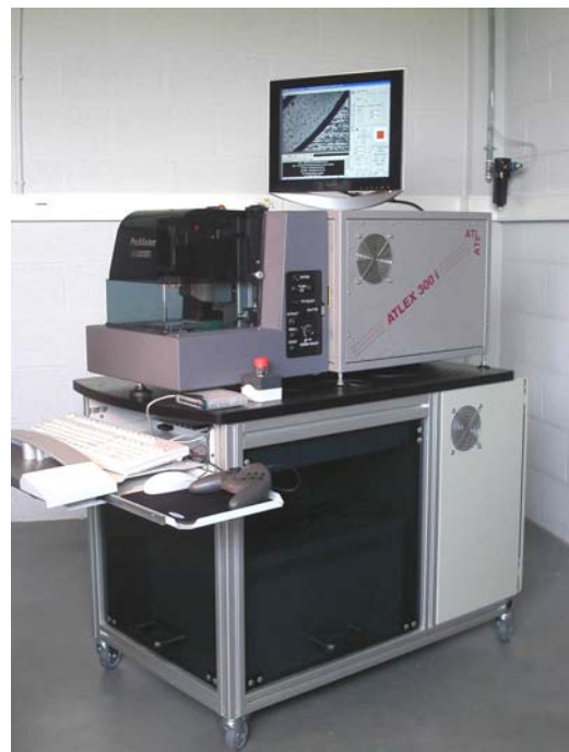
ProMaster turnkey workstation includes chariot with integrated gas cabinet and operator console.
