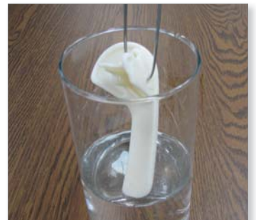
Figure 5: Sealing. Seal the part's surfaces by dipping in solvent.
