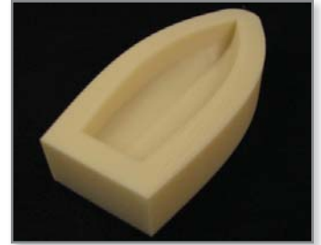
Figure 2: After support removal, the FDM mold can optionally be smoothed using the Smoothing Station offered by Stratasys.
