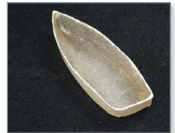
Finished Fiberglass part using an FDM mold.
