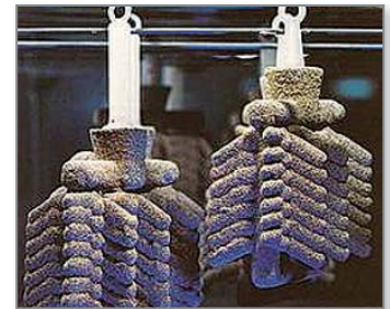
Figure 5: Parts on casting tree after shelling process.
