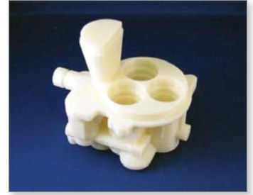
Figure 3: FDM pump body pattern, made from ABS-M30, is ready for shelling after sealing and sanding.
