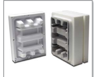
Figure 1: An example of Type 2 molding, which produces thinner products
