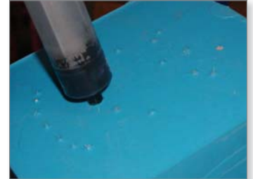
Figure 7: An alternative to gravity casting is to assist the pour by injecting the urethane with a large syringe.
