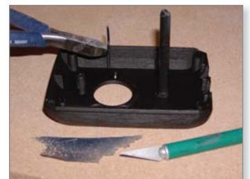
Figure 9: Trim the vents, gates and flash from the cast part with clippers, shears and X-Acto® knives.
