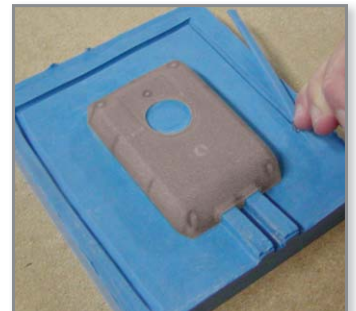
Figure 4: Using a round carving cutter, cut locator channels in the mold.
