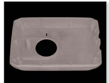
FDM pattern ready for use as an RTV mold.
