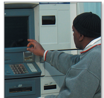
Image 3: Outdoor testing of an ATM prototype built with FDM components.
