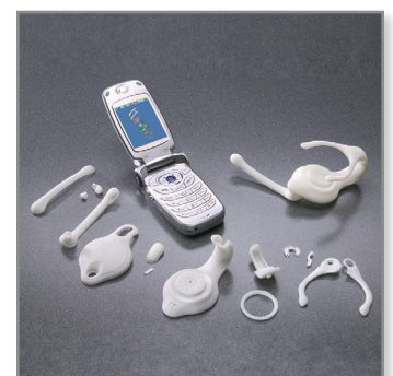
Image 3: Headset components were modeled in ABS plastic, using the FDM process.
