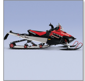
Image 1: Polaris avoided cutting two injection molding tools by using Fused Deposition Modeling (FDM) for a snowmobile carrier rack.
