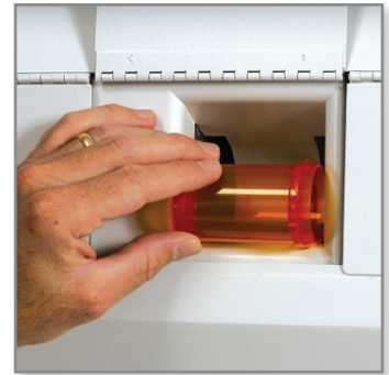
Image 4: Loading vials into the pill-dispensing machine. Each bezel allows only the correct vial type to be accepted.
