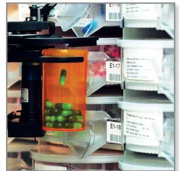
Image 5: A robotic arm picks up a vial, takes it to the dispensing cell for filling, then places it on a conveyor.
