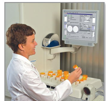
Image 6: After labeling, the conveyor moves the vial into a collated collection station
