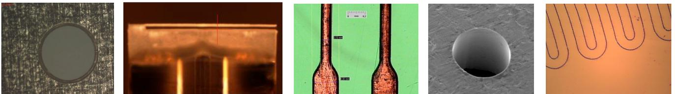
*Just a few examples of structures which can be produced by MM200-USP; stepped hole in s/s, cantilever in optical fibre(courtesy VUA), drossless cutting in Pt foil, drilling of polymer(courtesy Veld laser), scribing of SiN; consult Optec for process advice.*
