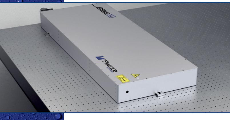
Jasper is a 1030 nm high-power femtosecond fiber laser, delivering pulses with energy up to 100 µJ and 60 W of average power. With truly monolithic all-fiber front-end this laser provides fast warm-up time, unprecedented long-term stability and hands-free operation. Contrary to free space laser amplifiers, fiber amplifiers ensure unbeatable beam pointing stability even in harsh environment.
